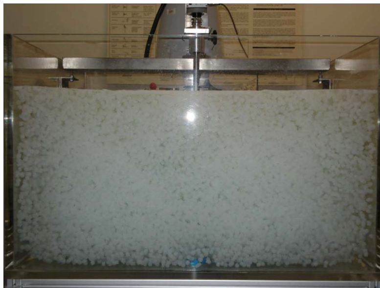
Fig.1. Side view of suspension experiment with plastic carriers
