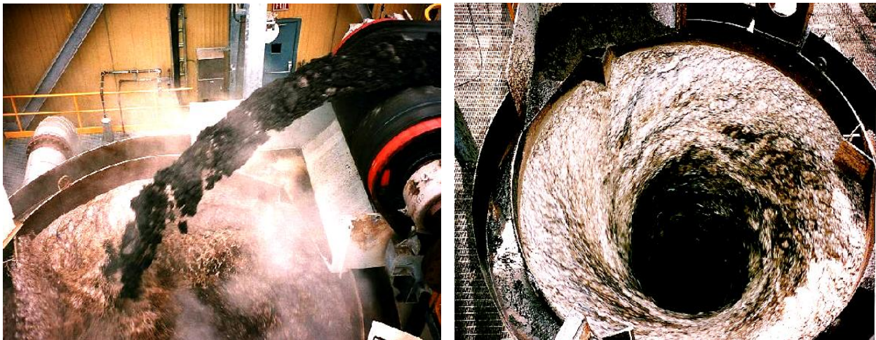
Figure 10 Swirling Action in a Cyclone Feeder [8, 9]
