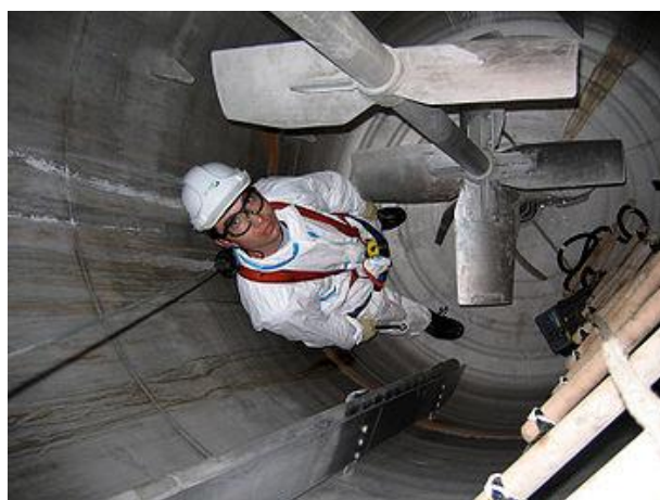
Figure 1. An industrial-size stirred reactor with multiple impellers and baffle 4
